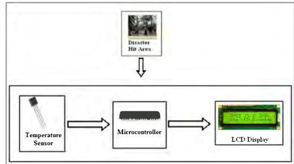
Figure2. Design of proposed system
