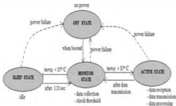
Figure 6. State Transition Diagram
