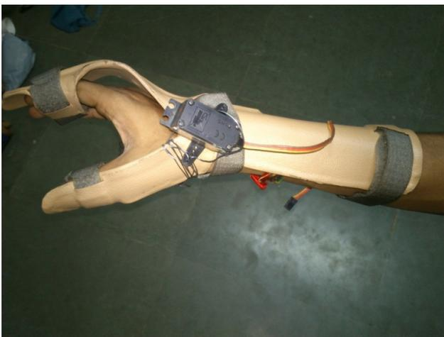
Fig.1a. Prosthetic arm with a servo motor placed on forearm.
