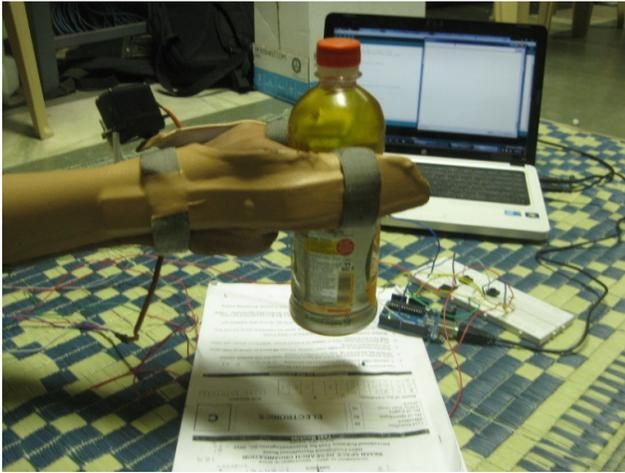
Fig.7. Arm holding an object and circuit setup
