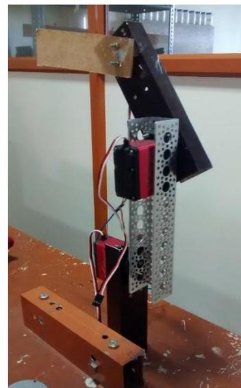
Figure 11. The 3 DOF robotic arm used for this experiment.
