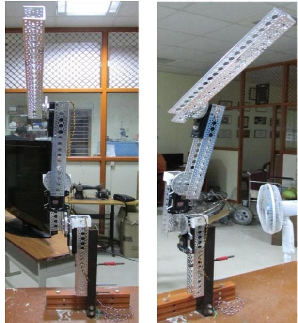
Figure 5. The robotic arm constructed using aluminum links, mounted in the laboratory.
