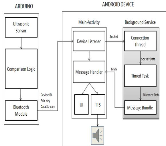
Fig.4. Arduino-Android Interfacing
