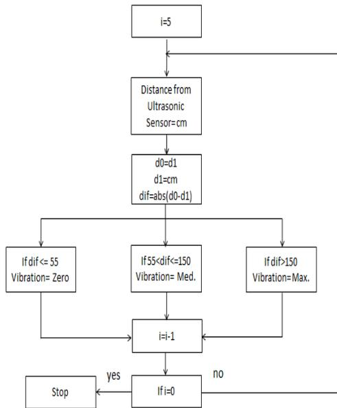
Fig.3. Flowchart for Moving Obstacle Detection
