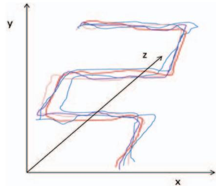
Fig. 6. Paths of the robot while climbing up
