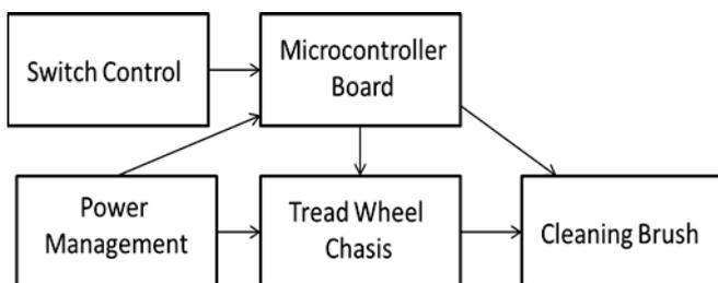
Fig. 2. General system architecture of the design
