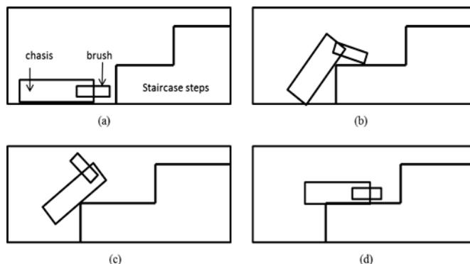
Fig. 2. Various positions of the robot while climbing up
