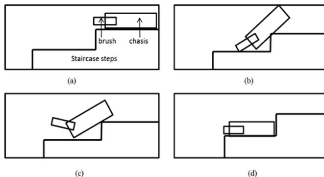
Fig. 3. Various positions of the robot while climbing down
