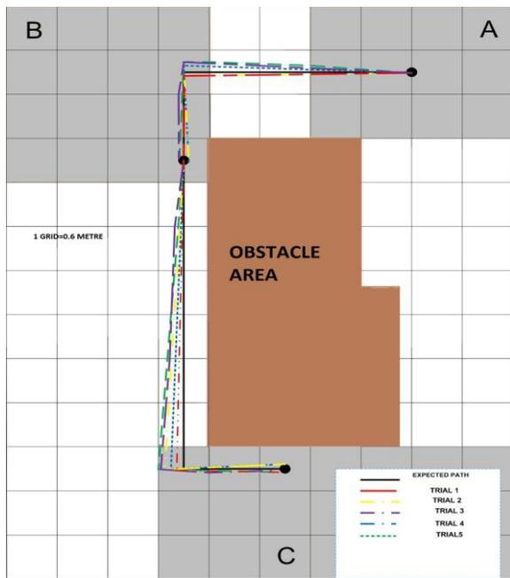
Fig. 9a. Plots showing expected path and different paths obtained for some of the trials using Arduino UNO
