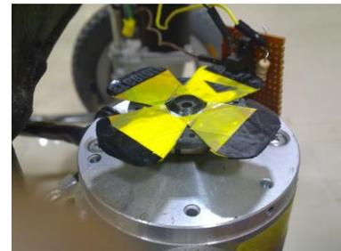
Fig. 4. Rotational encoder disc with pulse counting circuit
