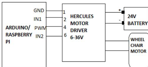
Fig. 7. Port Connections between Arduino or Raspberry Pi, Motor Driver and Motor
