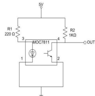
Fig. 6. Circuit Diagram of Rotation Encoder
