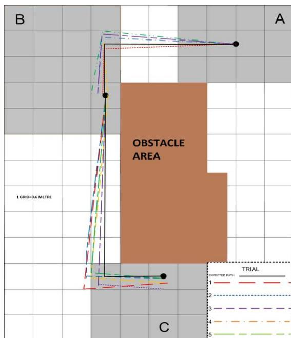
Fig. 9b. Plots showing expected path and different paths obtained for some of the trials using Raspberry Pi
