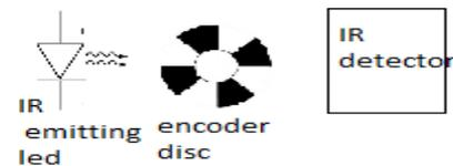
Fig. 5. Working principle of Rotation Encoder
