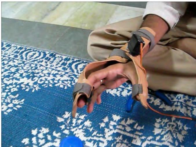
Fig.1a. Prosthetic arm with a servo motor placed on forearm
