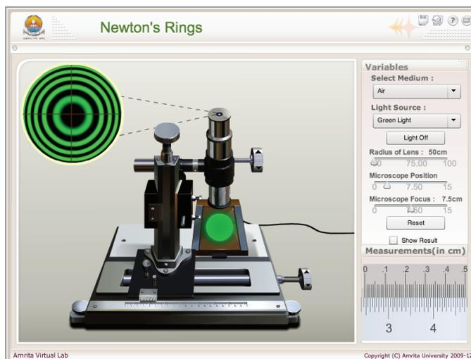
Fig. 2 Newton's Ring Apparatus
