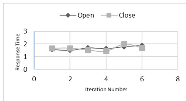
Fig. 7. Response time of the device for the commands using voice recognition module.
