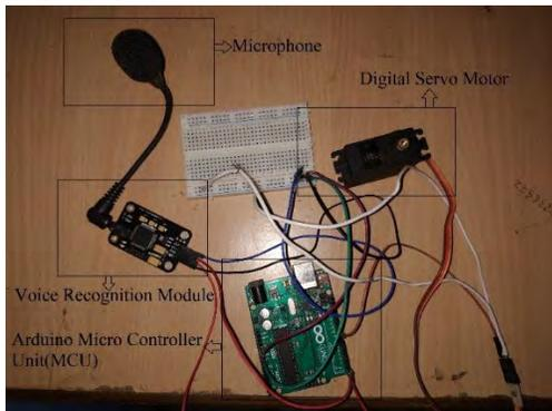
Fig. 4. Control Circuit with mike, MCU, voice recognition module and servo motor.
