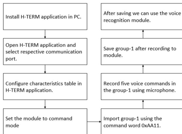
Fig. 2. Procedure for configuring Voice Recognition Module
