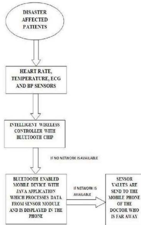
Figure. 2. Algorithm of the system
