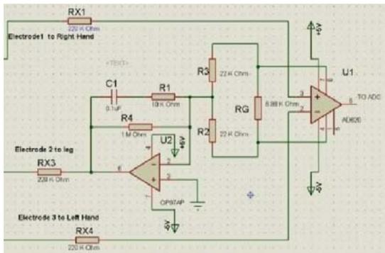
Figure. 1 ECG Sensor circuit
