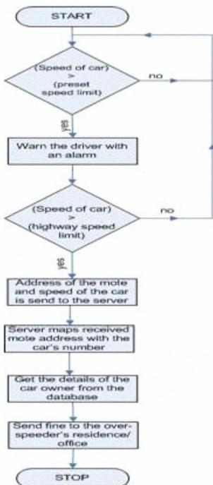
Fig.4 Over speed Detection Algorithm
