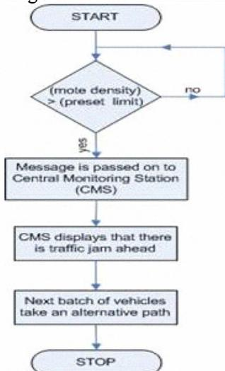
Fig.3 Traffic Routing Algorithm
