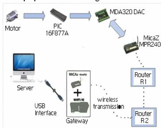
Fig. 5 Vehicle Speed Monitoring and Traffic Routing System(VSMTRS)
